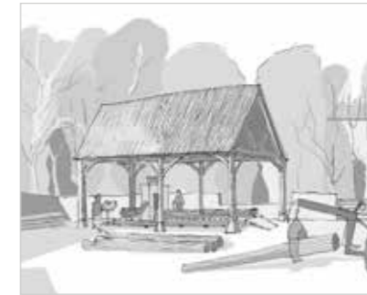
The milling and timber storage barns. Two new structures, made from Westonbirt wood, will allow timber to be milled and stored onsite.
